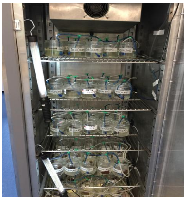
Figure 2.2. One of the experimental set-ups in the incubators showing the arrangement of the jars with one A. aquaticus in each jar exposed to experimental media (Solvent control (SCTR), Low treatment (LT) & High treatment (HT))
