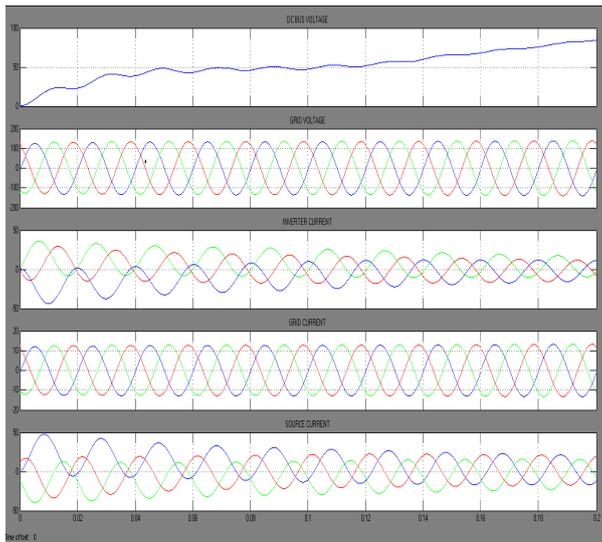
Fig. 5. Output of the PMSG based wind turbine system using back to back converters
