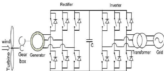
Fig. 3. Circuit diagram of back to back converter
