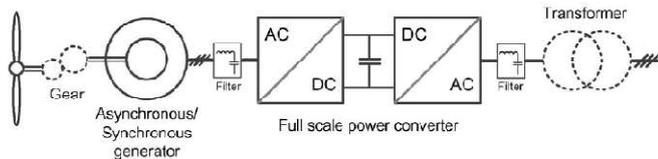
Fig. 1. General diagram of wind turbine system
