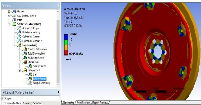
Fig. 5.7. Area of minimum stress fatigue safety factor
