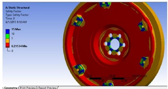
Fig. 5.4. Area of minimum stress fatigue safety factor
