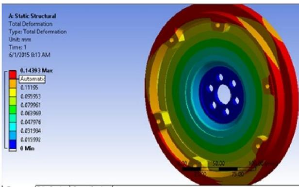
Fig. 5.1 Static structural results on flywheel total deformation
