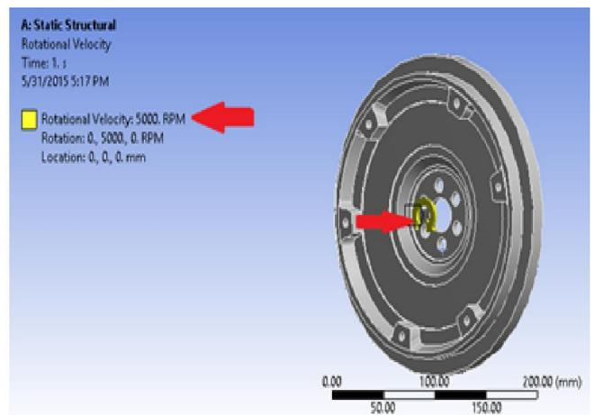
Fig. 4.3. Static loading conditions
