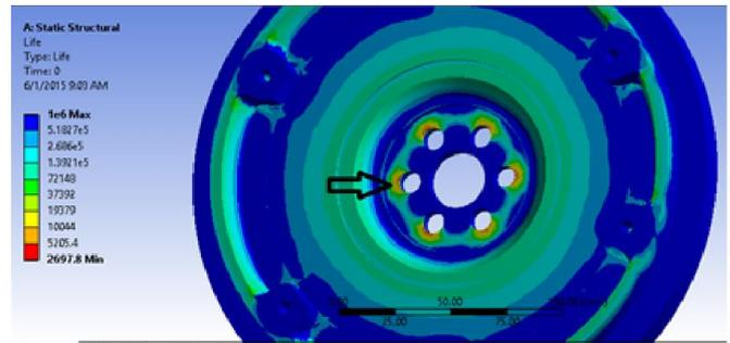
Fig. 5.3. Area of minimum stress fatigue life
