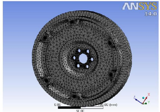
Fig. 4.2. Meshing in global flywheel model
