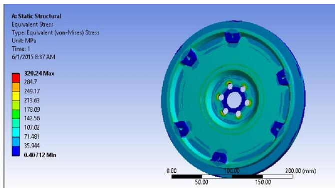
Fig. 5.2. Area of maximum stress on flywheel
