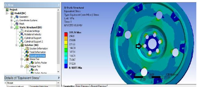
Fig.5.9 Maximum Von- stress on four circular cut flywheel disk after 10000 RPM
