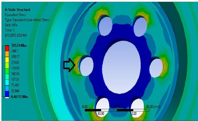
Fig. 5.5. Stress distribution in flywheel casing due to impact loading
