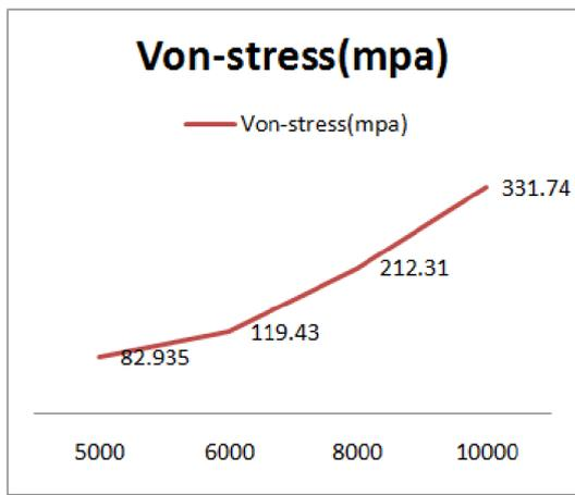
Fig. 5.10 Fatigue Stress Vs. RPM
