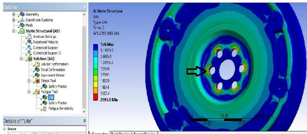
Fig. 5.6. Area of minimum stress fatigue life
