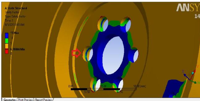
Fig. 5.3. Minimum factor of safety for static analysis
