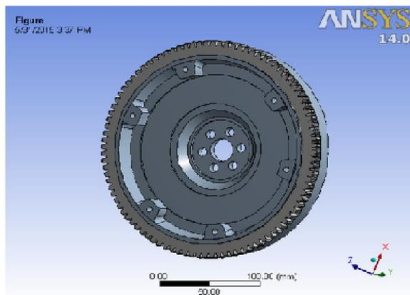
Fig. 4.1. Solid model of flywheel
