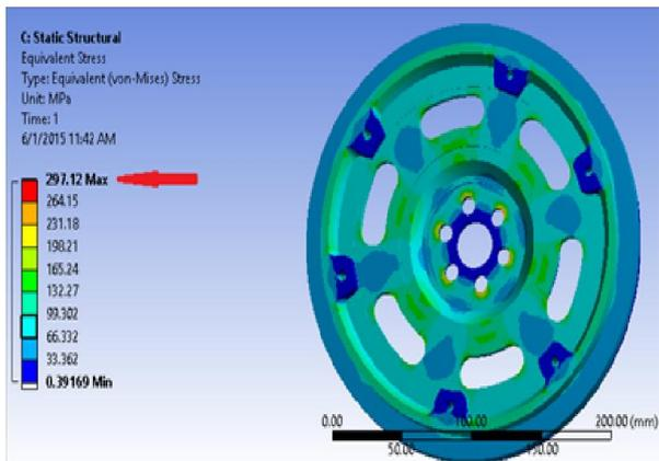
Fig 5.11. Maximum Von- stress on six cut slot flywheel disk after 10000RPM
