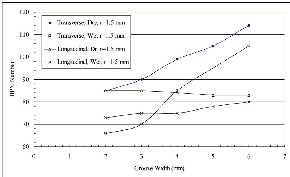
**Figure 6. British pendulum measurements for longitudinal and transverse rounded grooved surfaces with variable groove width, constant groove spacing and constant groove depth**
