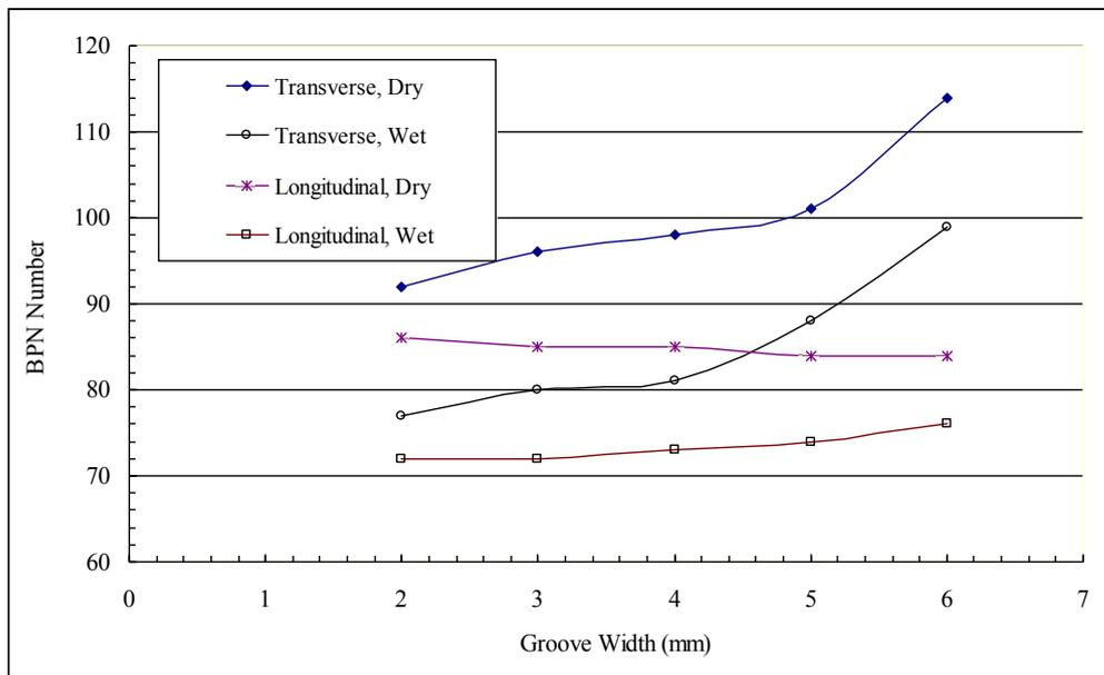
Figure 4. British pendulum measurements for longitudinal and transverse grooved surfaces with variable groove width, constant groove spacing and constant groove depth.
