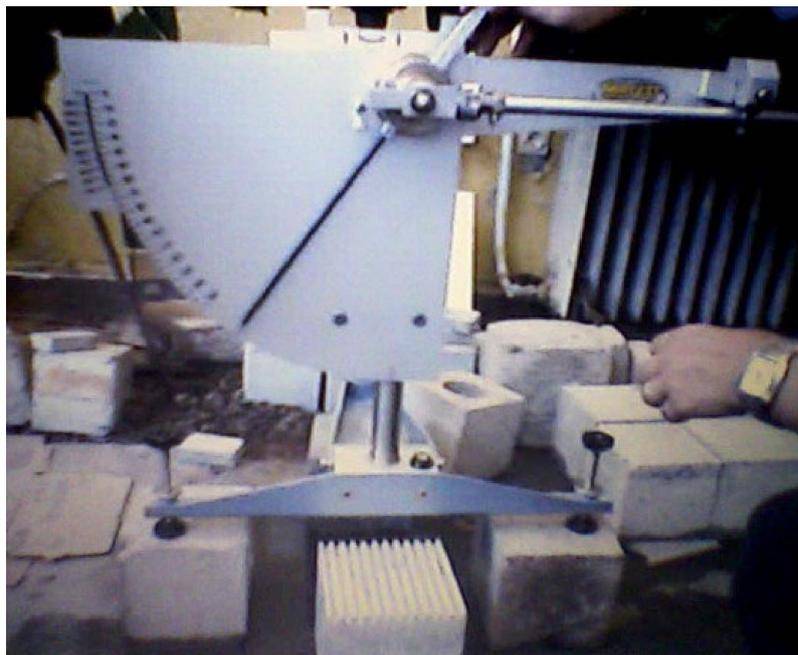
Figure 2. British Pendulum Testing on transverse grooved surface
