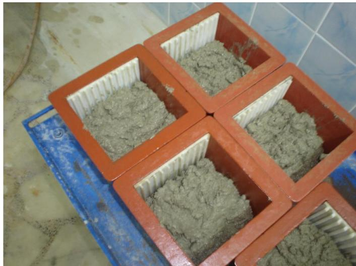
Figure 3. Plastic plates are on the side of the sample cubes
