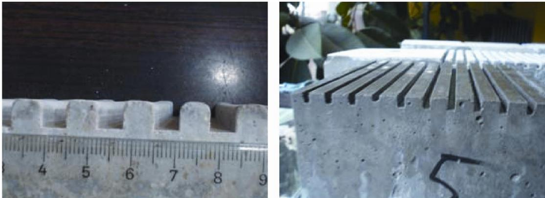
Figure 1. Grooves with rounded and sharp corner
